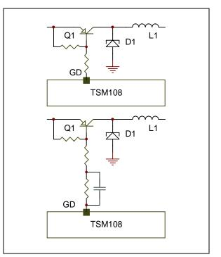
The most immediate way to choose from a P-channel MOSFET or a PNP transistor is to consider the ratio between the output power of the application and the expected components price: the lower the power, the more suitable the PNP transistor is; the higher the power, the more suitable the P-channel MOSFET is. As an example, for a DC/DC adaptor built for 12V/6V, the recommended limit to choose from one to the other is situated around 200mA.
