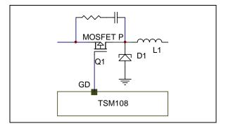
The RC components should realize a time constant corresponding to one tenth of the switching time constant of the TSM108 (i.e. in our example, the oscillator frequency is set to 10 $\mu$ s corresponding to 100kHz, therefore, the RC couple should realise a time constant close to 1 $\mu$ s).
